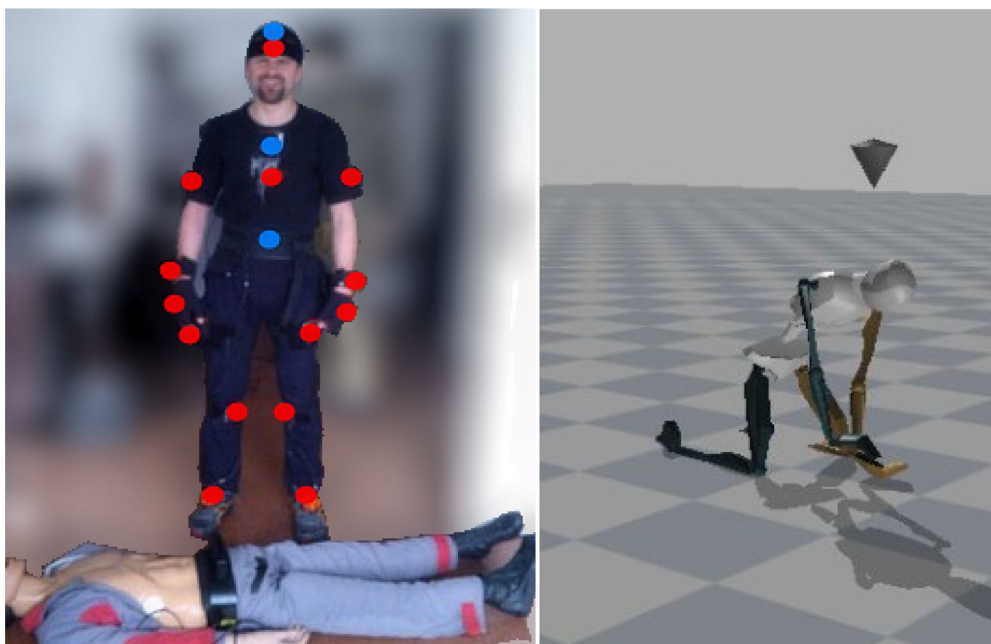
Fig. 2 The study participant wearing the Xsens MVN Biomech suit and Avatar—electronic imaging of the rescuer’s posture based on signals obtained from inertial sensors of the suit. Big, red point—front of the rescuer; big blue point—back of the rescuer (invisible)
