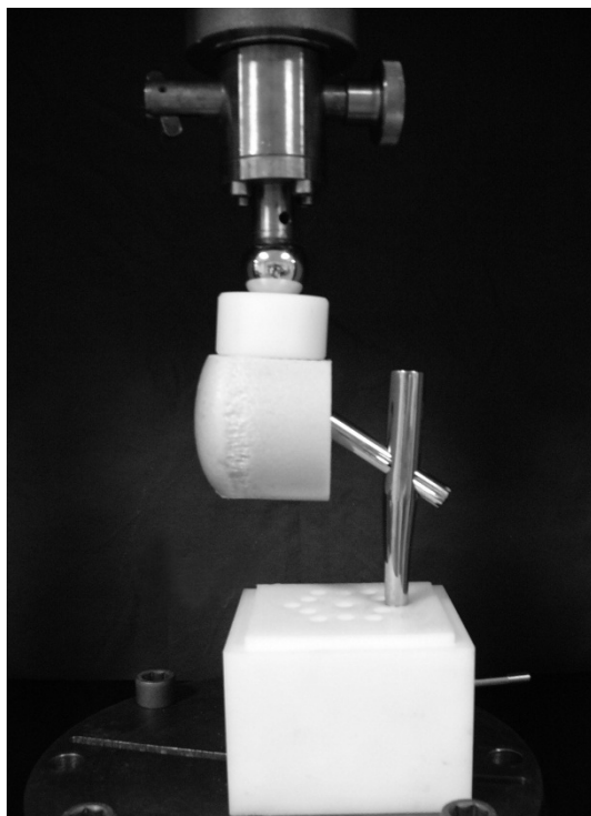
Fig. 4. Test arrangement mounted on MTS Zwick 1455.
